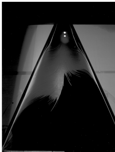
Fig. 2 Leeward-surface flow pattern visualized using different visualization fluids: a) oil-flow and b) fluorescent-dye/oil.
